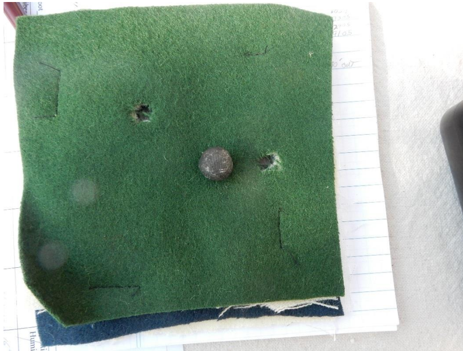
Figure 51. One of the cloth squares, 6x6 inch, used to simulate a Colonial era uniform clothing thickness. Two shots have passed through the cloth, and a recovered .626 diameter ball is shown next to the hole it created. Note: entry holes in cloth or tissue are often smaller than the bullet that created it due to the elasticity of the media.
