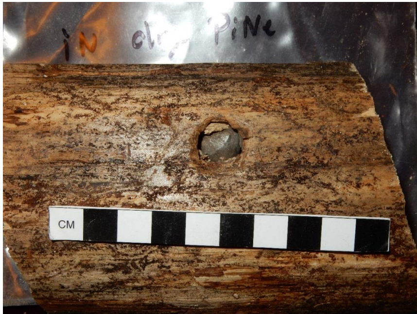
Figure 87. A .626 ball embedded \frac{3}{4} inch in a dry loblolly pine post. Note the deformation to the ball is moderate and would fall on the Bullet Deformation Scale as a 2. Pine is a relative soft media which is similar to tissue.
