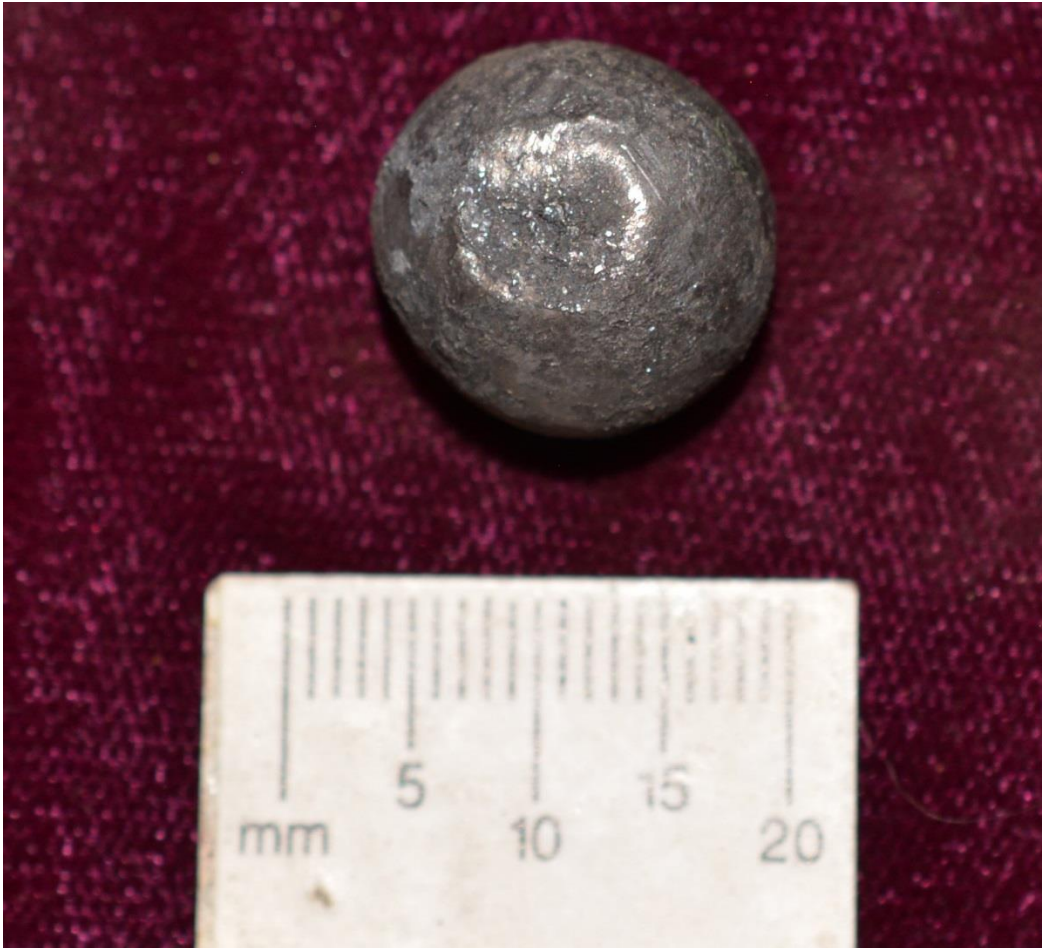
Figure 78. Typical denting and slight flattening caused by a ramrod head being forced against the ball during the loading of a muzzle loading firearm. There are different ramrod shapes for different firearms types and that data can be used to aid in identification of the type of gun in which the ball was fired.
