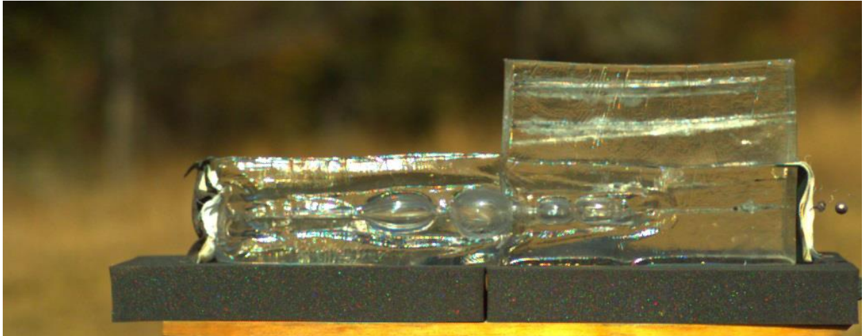
Figure 52. A .69 diameter ball fired from a British 1756 Long Land Pattern musket exiting 32 inches of gelatin. Note the initial wound cavity, bits of cloth in the wound cavity on the right and a larger piece of cloth exiting the block behind the ball.
