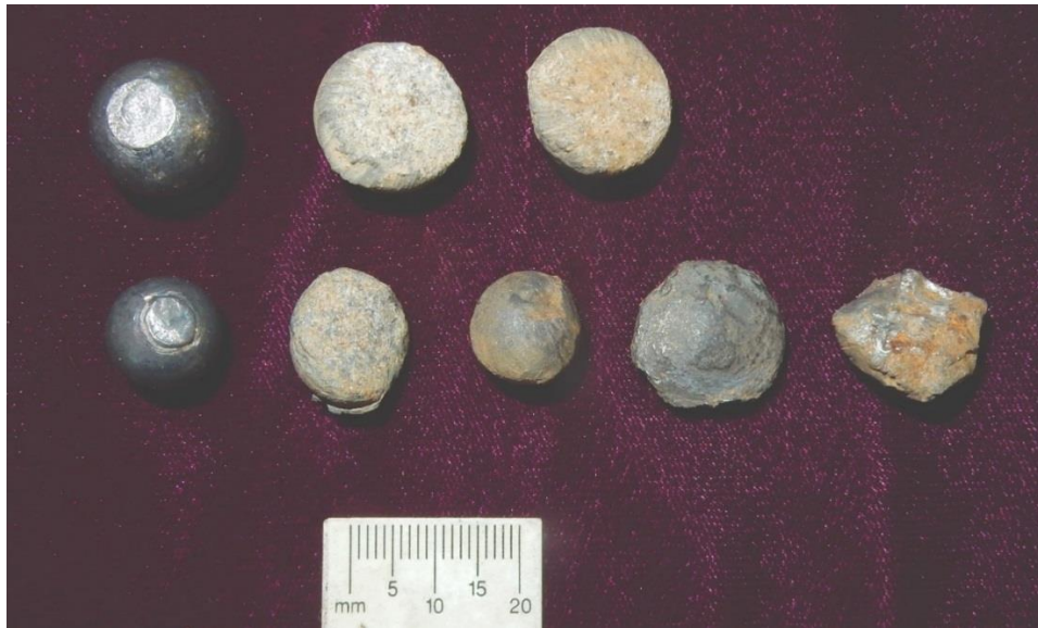
Figure 66. Top row, Unfired 0.626-inch ball, fired 0.626 ball at 1205 f/s and found in sand and soil backstop, fired 0.626 ball at 1215 f/s which nicked the target frame post and was found in the sand and soil backstop. Bottom row, Unfired 0.520-inch ball, fired 0.520 ball at 1215 f/s that hit oak palisade paling and ricocheted back into sand and soil backstop, fired 0.520 ball at 1250 f/s which hit a pine palisade paling and ricocheted back into sand and soil backstop, 0.520 ball at 1240 f/s that struck an oak palisade paling and fell to the ground below the fence, and 0.520 ball fired at 1285 f/s that went through a 4x4 pine target frame upright and was recovered in the sand and soil backstop. All balls found at 100 yards.
