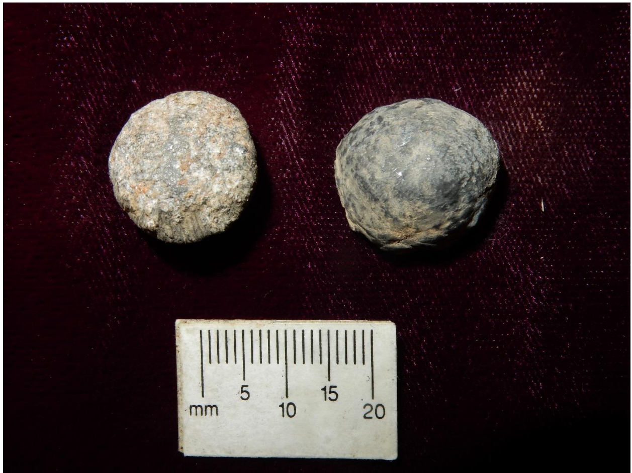
Figure 76. Two fired balls with significant impact scarring as well as impact deformation. The left ball shows significant flattening and the right ball also shows significant deformation. The left ball is scored at 3 and the right ball could be scored a 2.5 on the Bullet Deformation Index.
