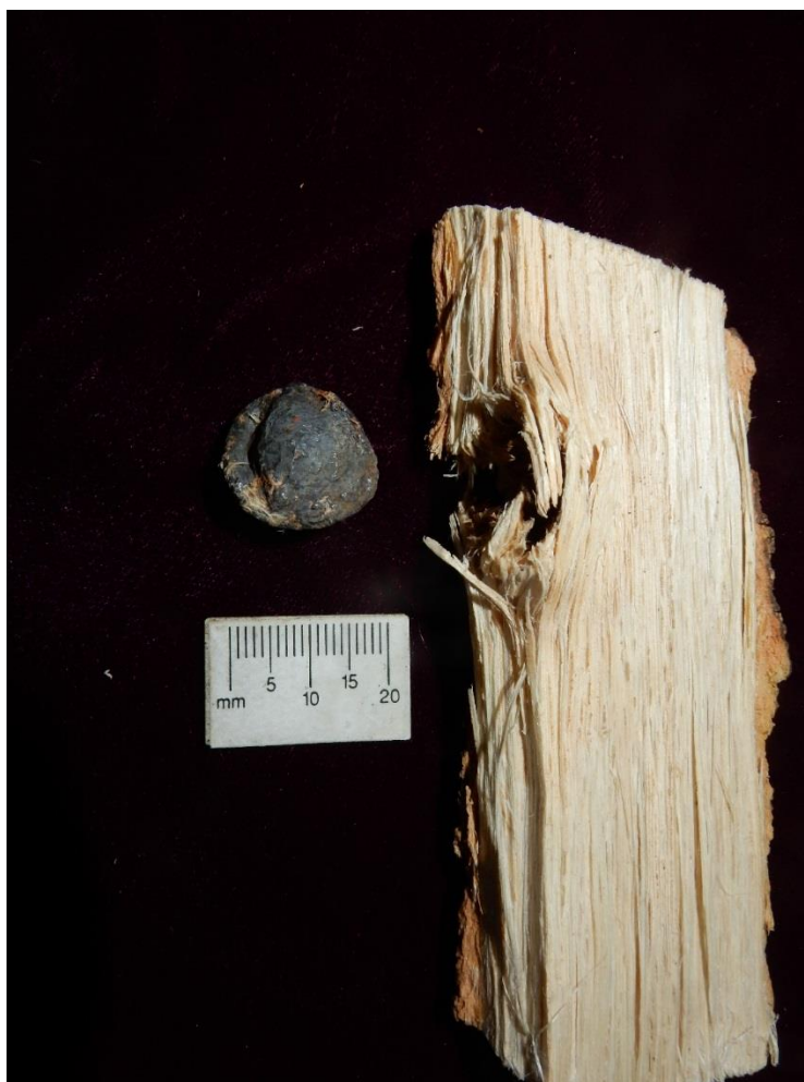
Figure 89. The .580 ball removed from the dry green oak. The ball is significantly deformed having hit at a higher velocity into a hard wood media. The bullet deformation is a 3 on the Bullet Deformation Scale.
