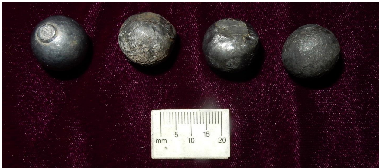
Figure 61. Unfired. 0.69-inch ball, 0.69 ball fired at 600 f/s that struck ground surface at 100 yards, 0.69 ball fired at 630 f/s that struck a wood table, foam, and ballistic gel at 25 yards and was collected laying on the foam at the back of 32 inches of ballistic gel, and a 0.69 ball fired at 630 f/s that was captured in the ballistic gel at 25 yards after passing through 28 inches of gel. Note fabric impression on second and fourth balls.
