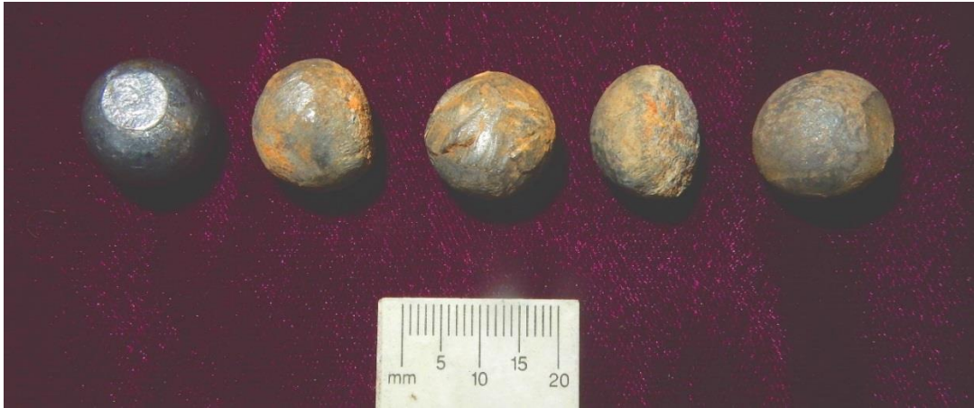
Figure 64. Unfired 0.626-inch ball, fired balls l to r fired at 905 f/s, 960 f/s, 960 f/s, and 1090 f/s. All balls recovered at 100 yards in sand and soil backstop. Note third ball from the left passed through a pine 4x4 target frame upright and the fourth ball from left also struck the edge of the pine target frame before embedding in the backstop.
