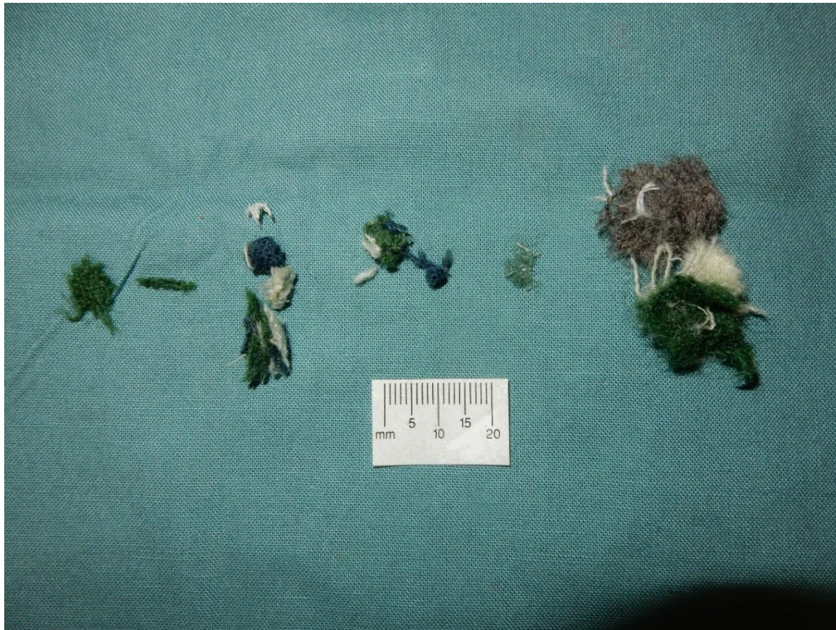
Figure 59. Fragments of fabric recovered from gelatin wound tracks. L to R. recovered from entry site 4 inch in, 12 inches in, 12 to 14 inches in, 14 to 16 inches in, 15 to 16 inches in and 30 inches in. In a real wound track the fabric would be sources for infection and sepsis, a known issue in eighteenth century medicine.
