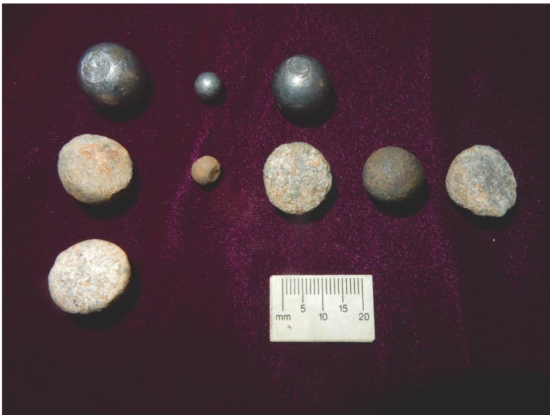
Figure 65. Left column, unfired 0.626-inch ball, fired 0.626 balls at 1110 f/s and 1175 f/s, both found in sand and soil backstop. Second column, unfired 0.282 buckshot and fired 0.282 buckshot at 1110 f/s found in sand and soil backstop. Third column, unfired .580-inch ball and fired 0.580 ball at 1135 f/s found in sand and soil backstop. Fourth column, 0.580 ball fired at 1155 f/s, and Fifth column, 0.580 ball fired at 1170 f/s and found in soil and sand backstop. All balls recovered at 100 yards.
