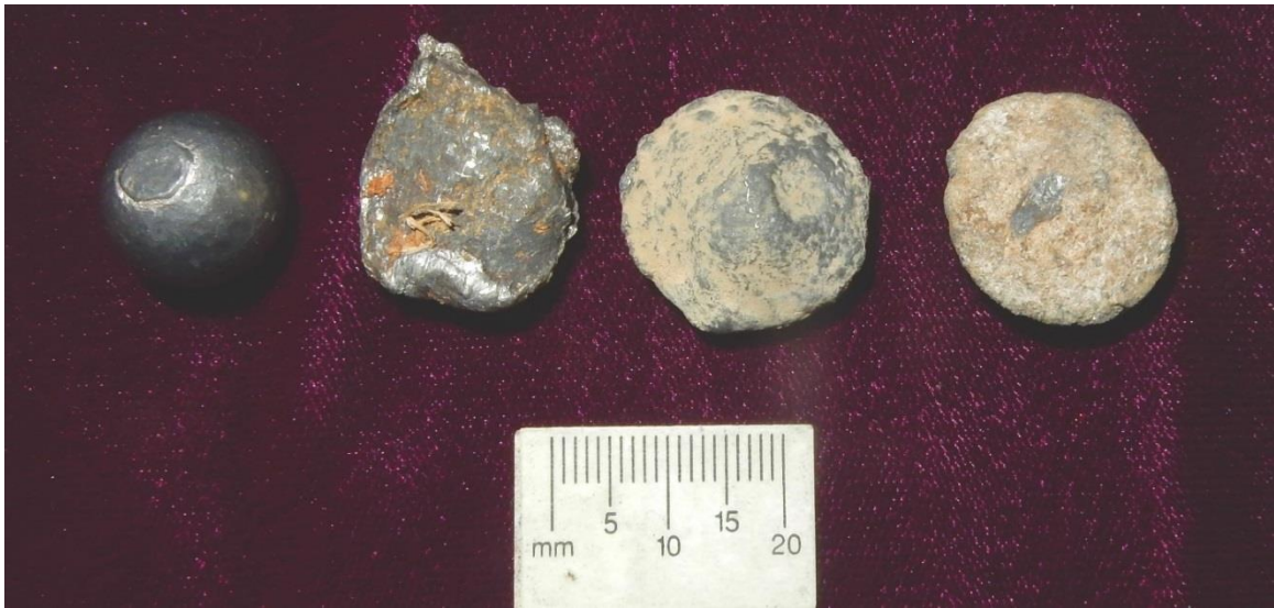
Figure 68. Unfired 0.580-inch ball and fired balls, second – fired at 1415 f/s and struck oak palisade paling and found in sand and soil backstop below fence, third – fired at 1435 f/s and found in sand and soil backstop, fourth – fired at 1480 f/s and found in sand and soil backstop. All balls recovered at 100 yards.
