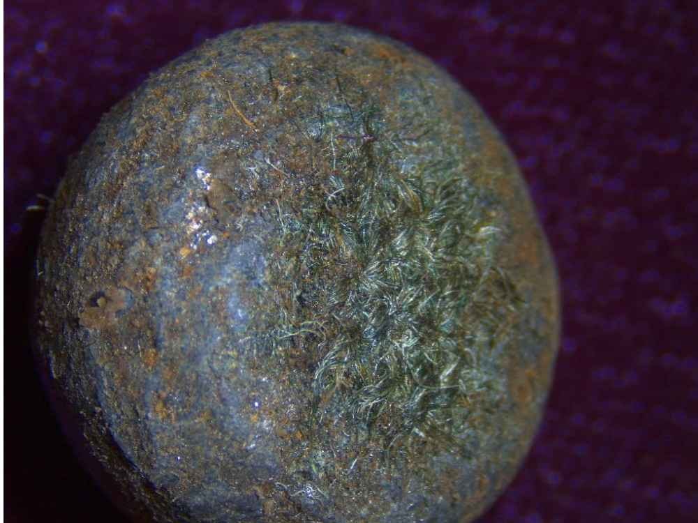
Figure 85. A 20x magnification of a ball fired from the 1763/66 French musket with fabric still adhering to its surface after passing through the simulated uniform cloth and gelatin blocks.
