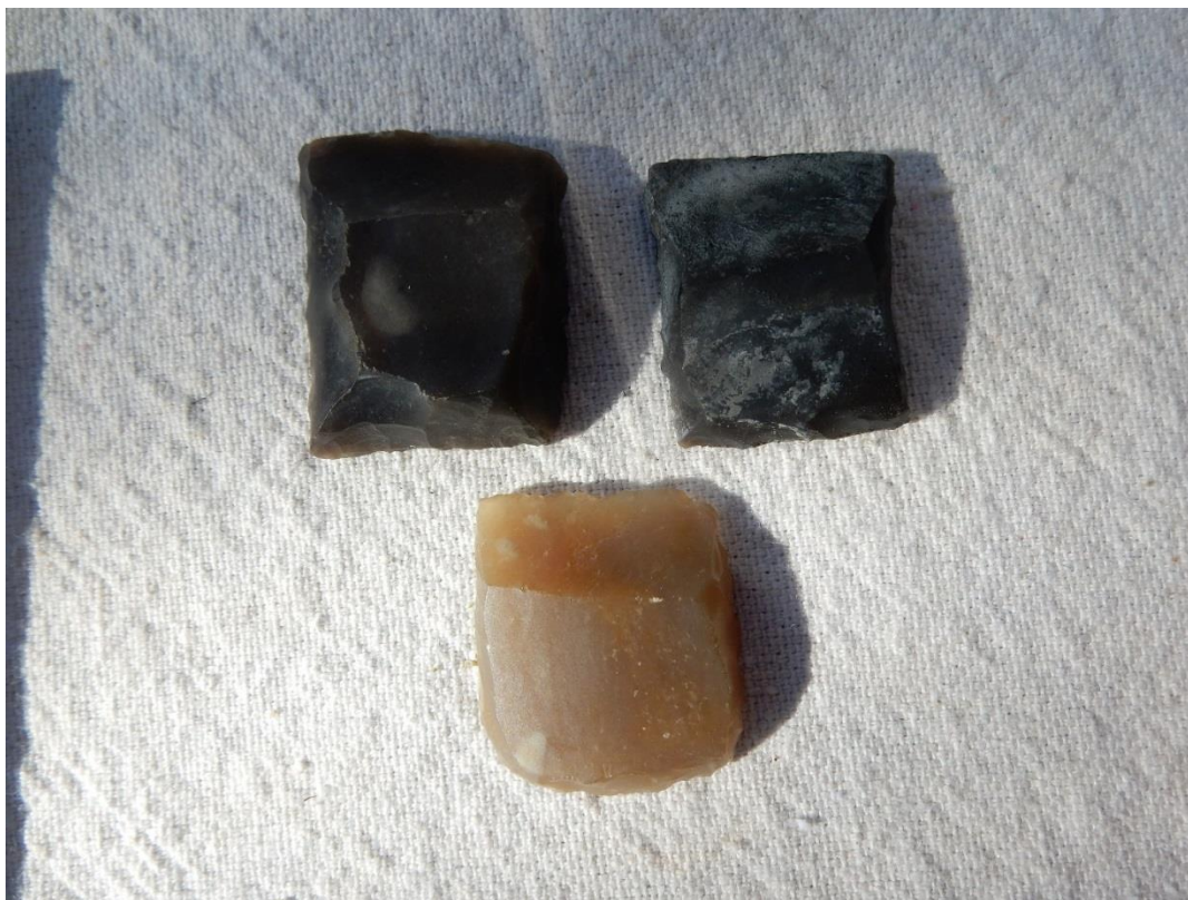
Figure 14. British and French gunflints used in the experimental firing. The top left is a British unused flint and the top right flint is fully expended. The bottom flint is a French style unused flint.
