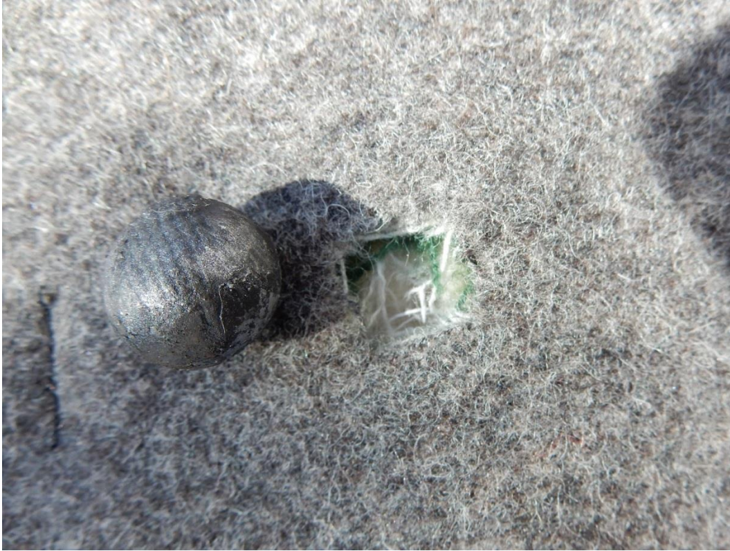
Figure 54. A fabric impressed .69 diameter ball fired from the British 1756 Long Land Pattern musket with 75 grains of powder at 25 yards. The fabric impressions resulted from passing through the simulated uniform clothing.
