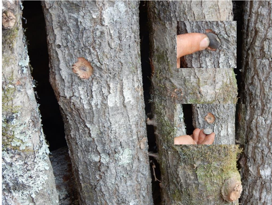
Figure 77. A Fowler .580-caliber ball hit on a live oak palisade piling with insets showing the complete flattening or mushrooming effect of a high velocity hit on a hard media. The muzzle velocity was 1240 f/s. The ball scores a 3 on the Bullet Deformation Index.
